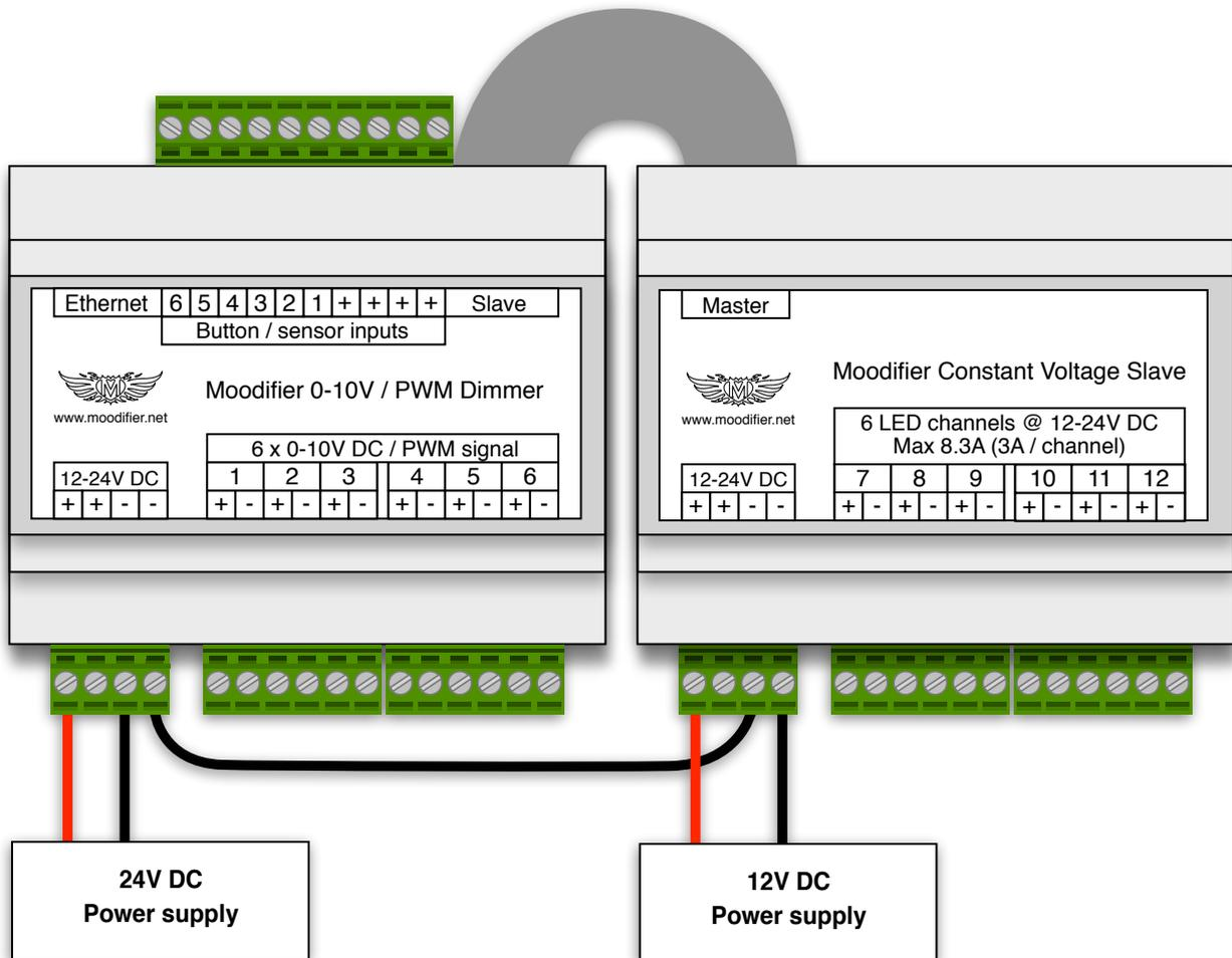
Interconnected Master and Slave units running at different voltages and power supplies with common grounding.
