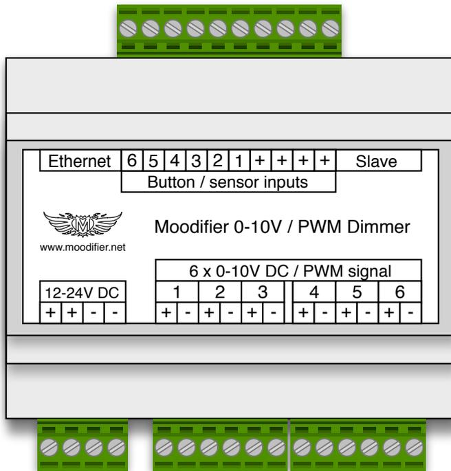
The DIN-rail mounted Moodifier Dimmer unit seen from above with connectors facing up/down.
