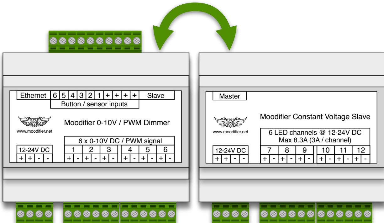
You can connect 2 types of slave units to the Moodifier Dimmer, a Moodifier Constant Current Slave unit or a Moodifier Constant Voltage Slave unit. This adds great flexibility when designing your lighting since it enables a wide range of options for both 0-10V and PWM controlled equipment as well as constant current and constant voltage based LED lighting and relays.
