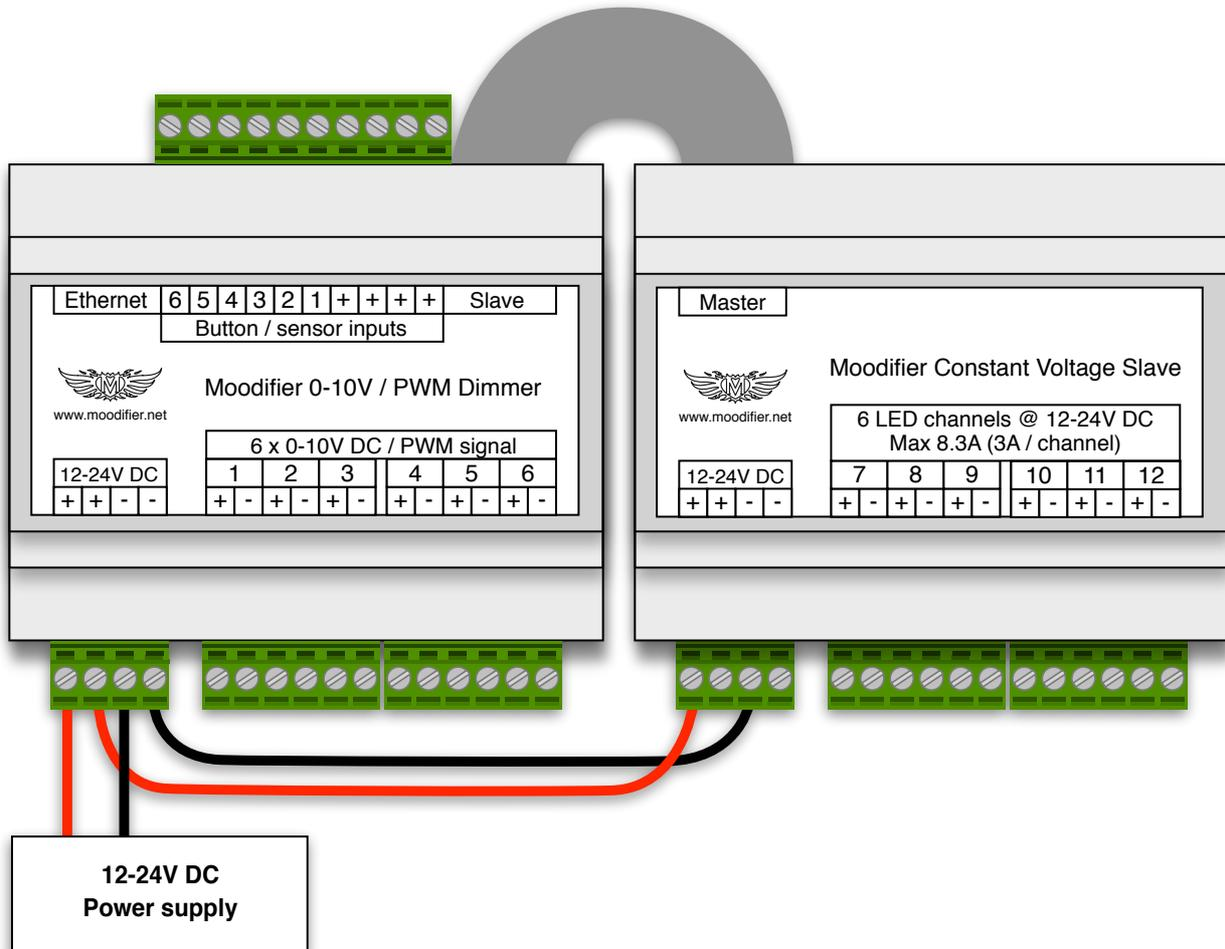
By putting a standard wall switch that cuts the power to the power supply you will get a master power on/off switch for the device. Use the Moodifier application to set the default light setting that is activated whenever the unit is powered up or after power failures.
